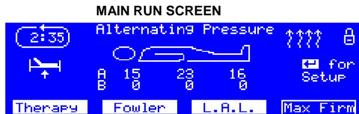
During normal operation, the following words appear above the four Menu Keys. Pressing a key results in the corresponding action.
